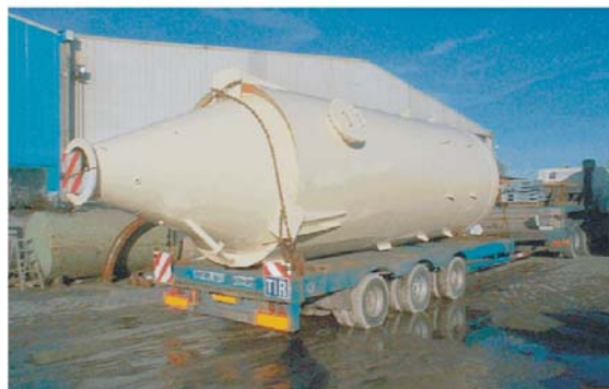
fig. 1 small silo built to contain explosion induced pressure rise
